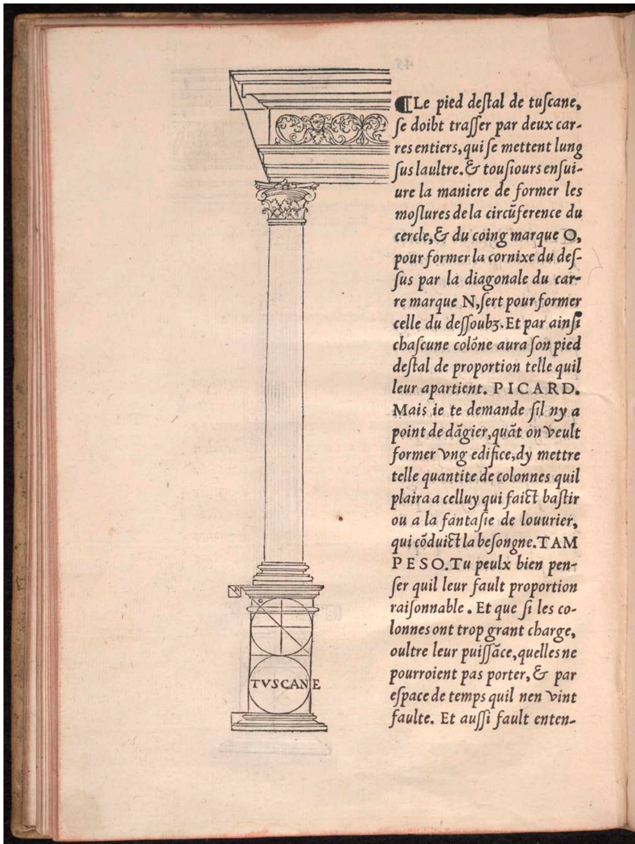
Fig. 9: French Anonymus, Raison d'architecture antique (Paris, before 1536), fol. 45 recto: Proportioning of the Tuscan (i.e. Composite) order. University of Virginia Library.
