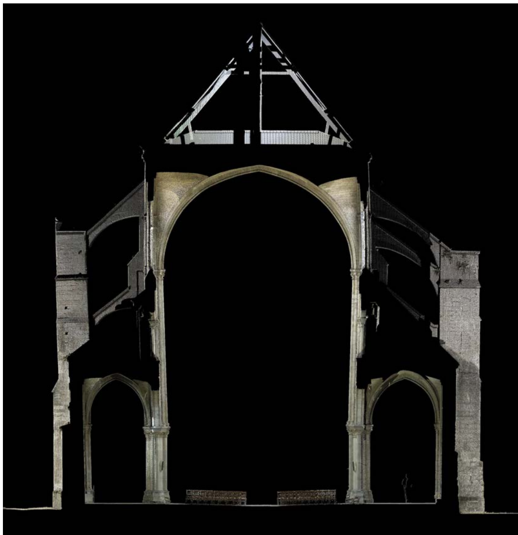
Fig. 7: Abbey church of Saint-Leu-d'Esserent, laser scan, June 2011: section through the nave. Image: Andrew Tallon.
