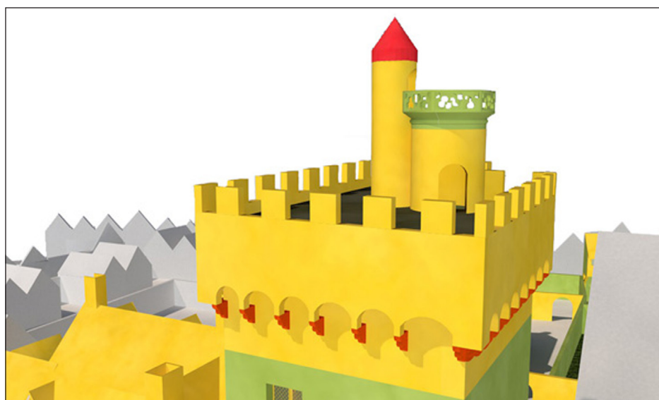
Figure 17: The rooftop of the tower with the panoramic roof and openwork parapet. Code: red = full hypothesis; orange = analogy; yellow = estimated reconstruction; light green = confirmed by one source; dark green = confirmed by multiple sources. Image created by Sanne Maekelberg.
