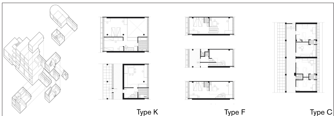
Figure 13: Narkomfin House proposal developed by Ginzburg and Milinis (1929–30): axonometric view of the cluster system and floor plans of types K, F, and C, built version. Graphics by Daniel Movilla Vega.
