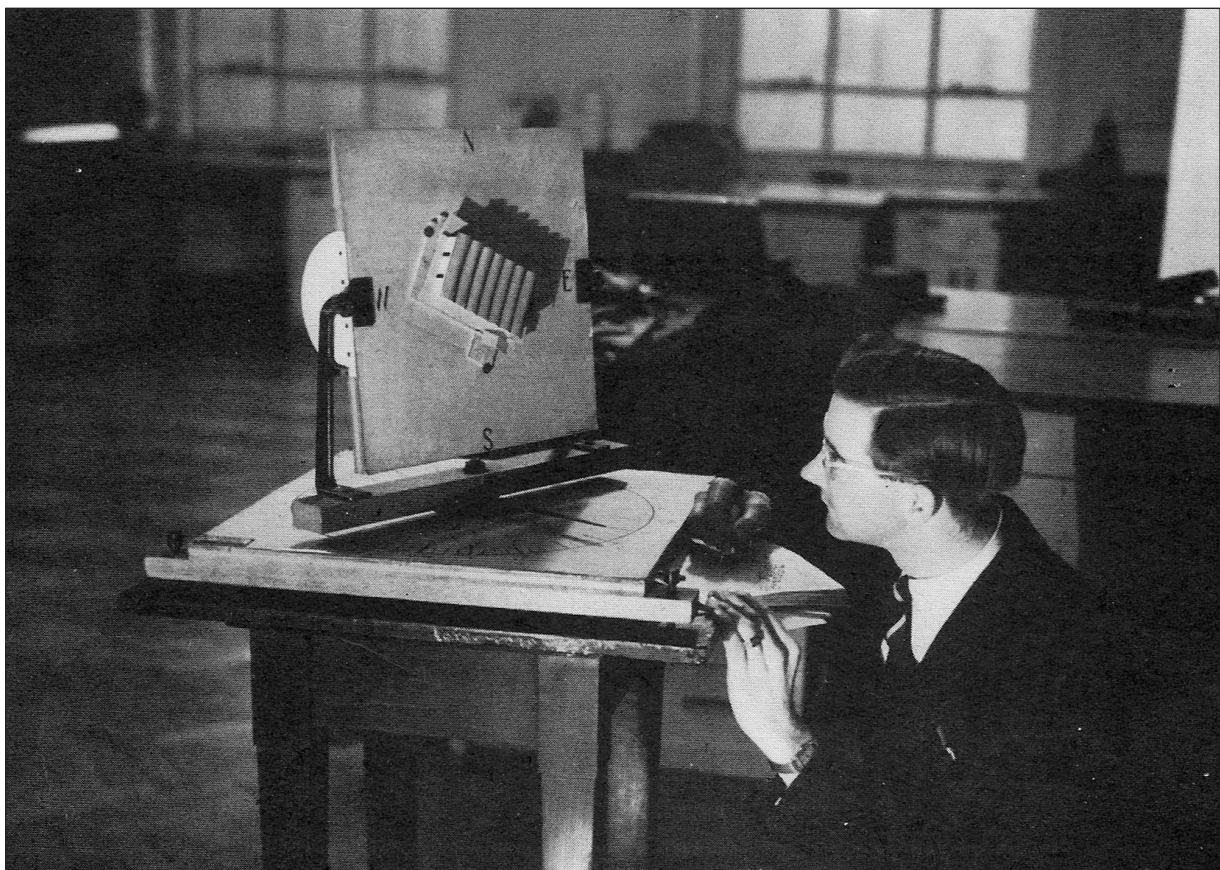
Figure 2: A researcher placing the model of the Dining Hall, designed by Maxwell Fry and Jane Drew, at University College, Ibadan, Nigeria, on a heliodon to study the effectiveness of the sun-shading. From Foyle (1953).
