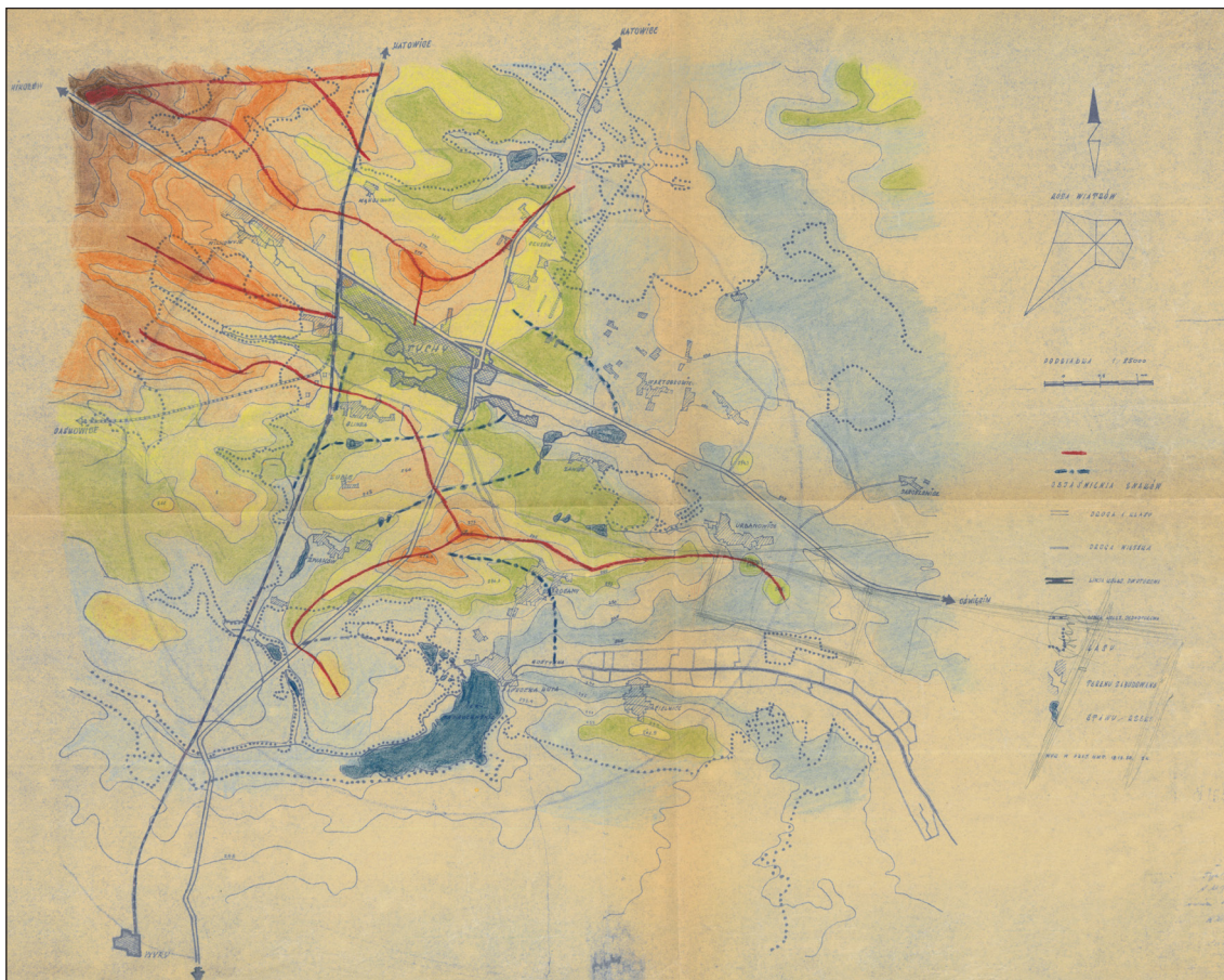
Figure 1: Map showing the planning conditions of the proposed city: topography, existing transport lines, village of Tychy to the north and Lake Paprocany to the south. Scale 1:25 000, ca. 1950. Collection of the Tychy City Museum.
